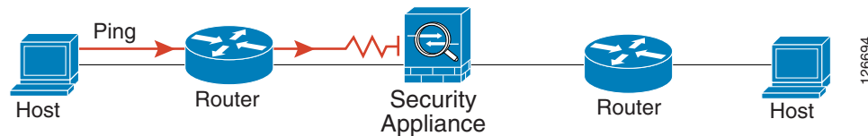
Figure 24-5 Ping Failure Because the ASA is Not Translating Addresses
